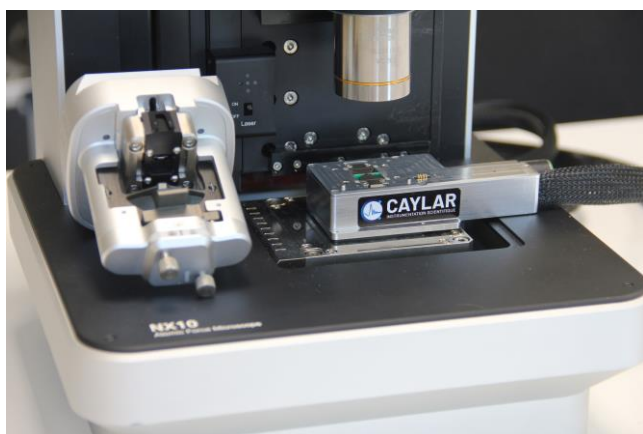
MFM Installed in a NX10 AFM (Park Systems)
